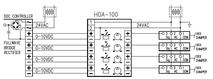
Terminal 2 of the HOA-100 is common to both input and output common (-) terminals. If being used with a controller that utilizes a full wave bridge rectifier in its power supply section (output common is floating or not connected to one side of AC input) an isolation transformer must be used to prevent damage to power supply section.
