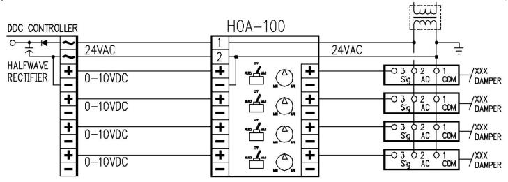
The HOA-100 was designed to provide hand-off-auto capability to DDC type controllers in controlling damper position. The HOA-100 can be used for Hand-off-auto operations in other applications. Terminal 2 of the HOA-100 is common to both input and output common (-) terminals. The same transformer can be used but polarity must be observed.
